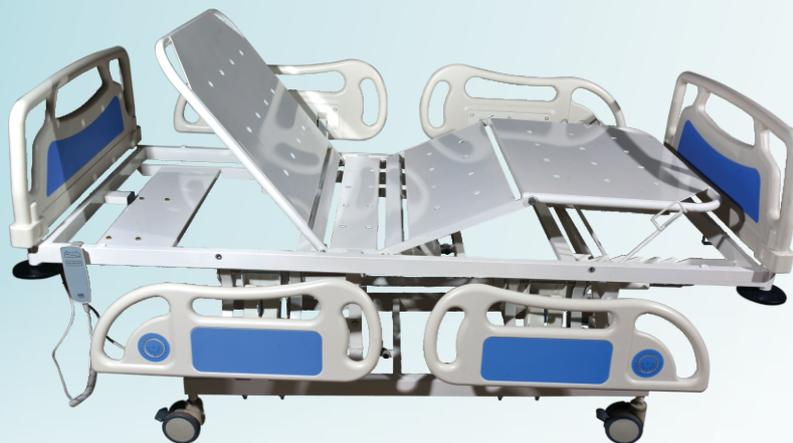
The C.R. sheet top is uniformly perforated in four sections with two electrical motors for back rest and height adjustment, two screw mechanism for trendelenburg, reverse trendelenburg and knee rest. Detachable ABS bows, IV stand and ABS railings. The entire structure is mounted on 125mm dia castor wheels – two with brake. Pretreated and powder coated.
