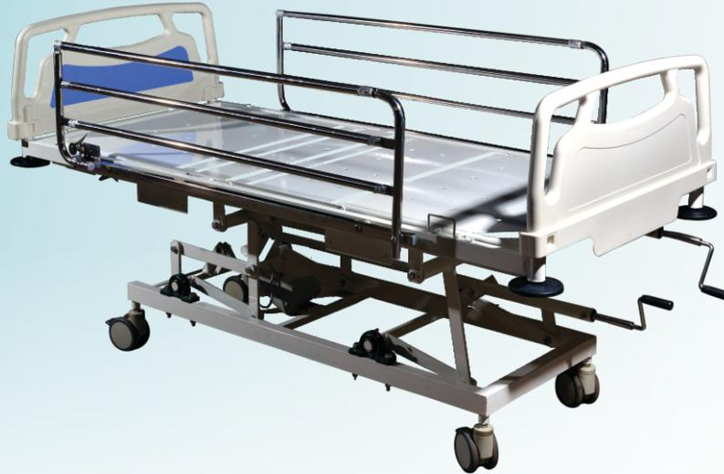
The C.R. sheet top is uniformly perforated in four sections for back rest, knee rest, trendelenburg, reverse trendelenburg and height adjustment, Detachable ABS bows, I.V. stand and S.S. railings (size: 1370 x 350mm). The entire structure is mounted on 125mm dia castor wheels – two with brake. Pre-treated and powder coated.
